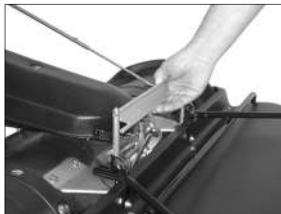
6) The debris container is locked.
