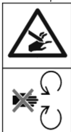
Do not open the protective equipment, risk of crushing
