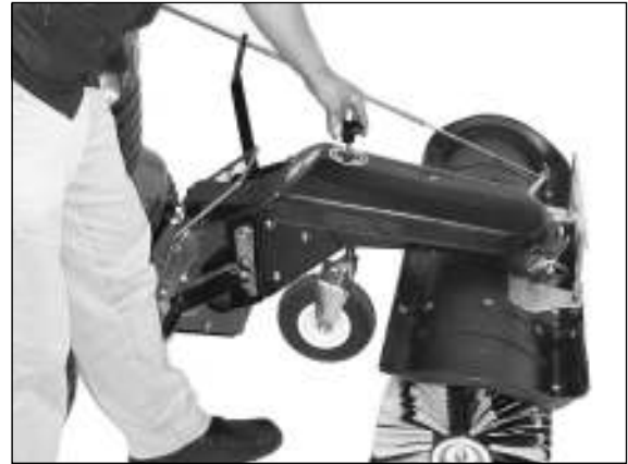
2) The height of the support wheel is adjusted by turning the ball handle.
