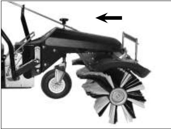
1) The ball handle for adjusting the brush pressure is located above the support wheel.
