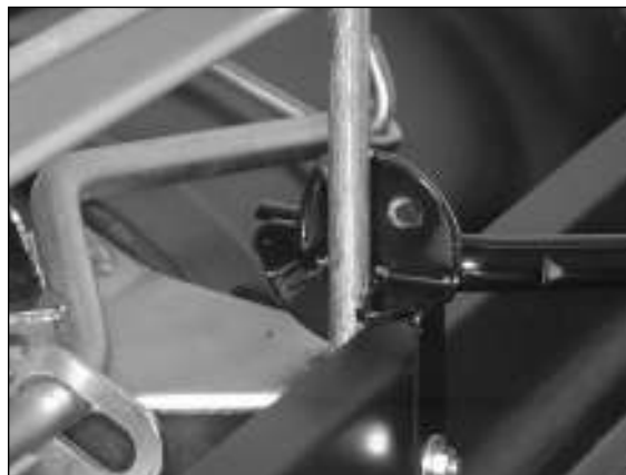
4) Debris container in the bottom position.
