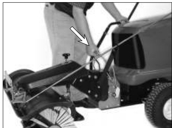
6) Push the coupler handle down at an angle.
