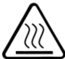
Caution: Hot surface
