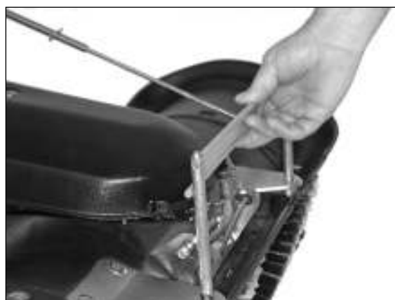
2) Locking mechanism turned backwards.
