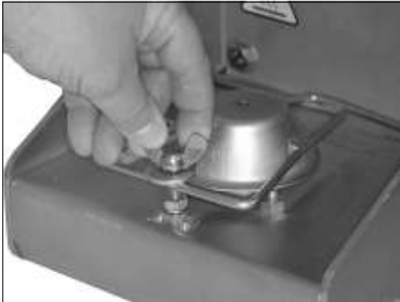
1) Undo the wing bolt on the quick-change mechanism guard.
