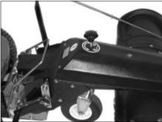
3) Optimal brush pressure: Lower the brush until it is just touching the floor. Then turn the handle all the way round three more times in an anti-clockwise direction (towards the (-) arrow).
